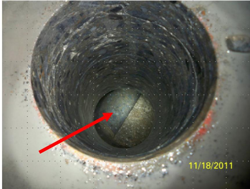
Figure 19: Core, 46 cm (18 inches) long, lying on its side at bottom of void beneath the PCC.
