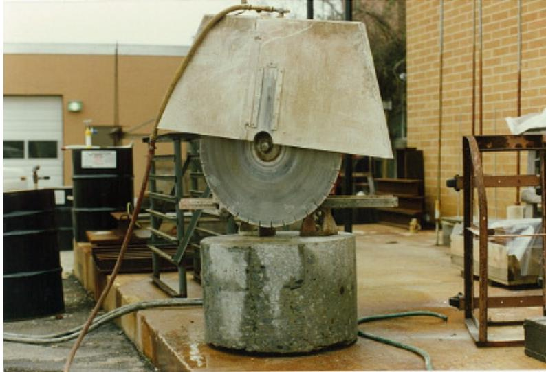
Figure 12: Set-up for sawing of LDC at laboratory.
