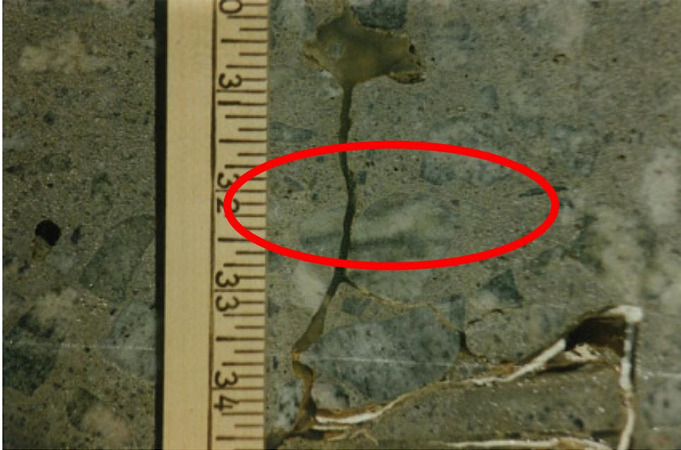
Figure 15: Note the vertical offset of 3 mm (1/8 inch) in the large aggregate. The styrofoam coffee cup (white material) was determined to be of no influence.
