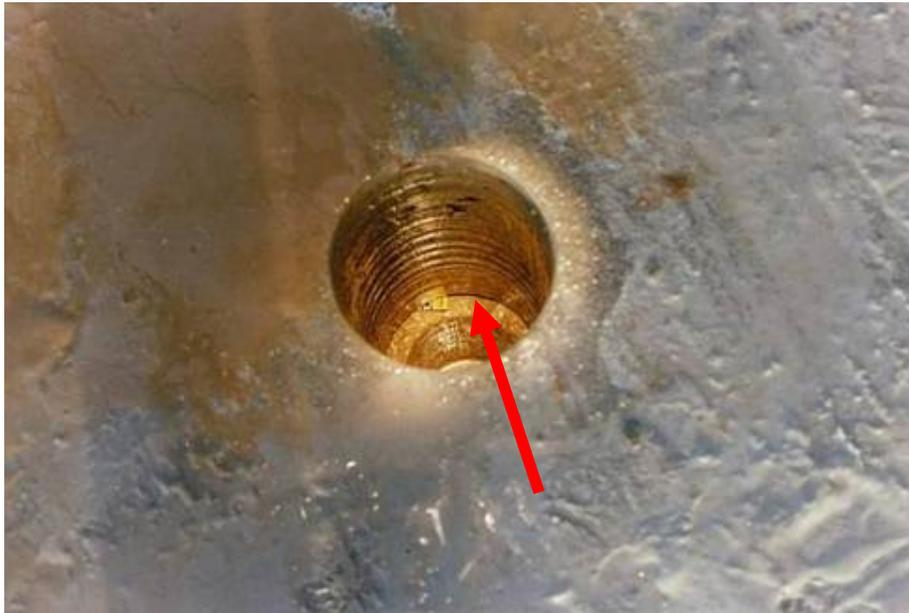
Figure 7: Void between PCC and CTB in the coring/boring in Slab 37B in Taxiway E.
