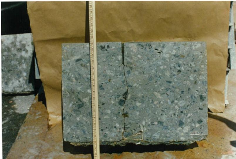
Figure 13: Slice of LDC with embedded dowel bar.
